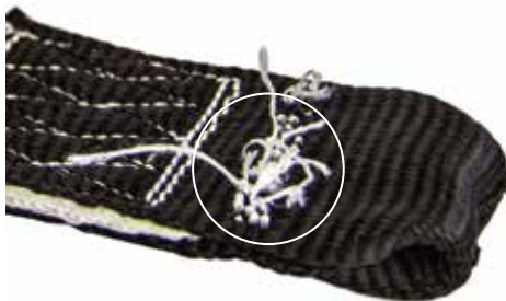
Broken/damaged indicator stitching - Immediately remove from service!
